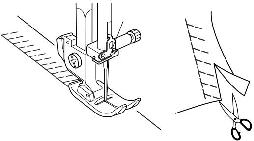
This stitch is ideal for 1/4" (0.6 cm) seams on knits or on medium to heavy weight woven fabrics where you want a narrow seam. It is also great for sewing spandex swim wear. Place the fabric to leave a 5/8" (1.6 cm) allowance.
