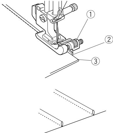
Fold a fabric wrong side together and Lower the needle into the fabric 0.1 – 0.2 cm inside the folded edge.
