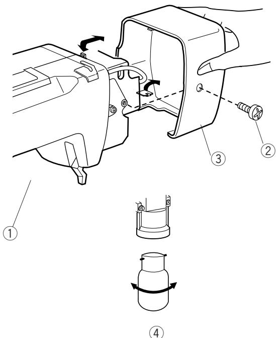
Remove the cap and screw. Remove the face plate.
