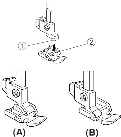
**A:** To sew the left side of the zipper, attach zipper foot with the right side pin.
