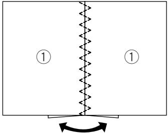
Place two layers of the fabric with the right side together. Seam along the edges with the straight stitch.
