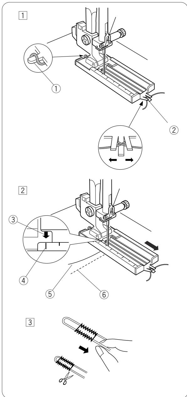
① With the buttonhole foot raised, hook the filler cord on the spur at the back of the foot. Bring the ends toward you under the foot, clearing the front end. Hook the filler cord into the forks on the front of the foot to hold them tight.
