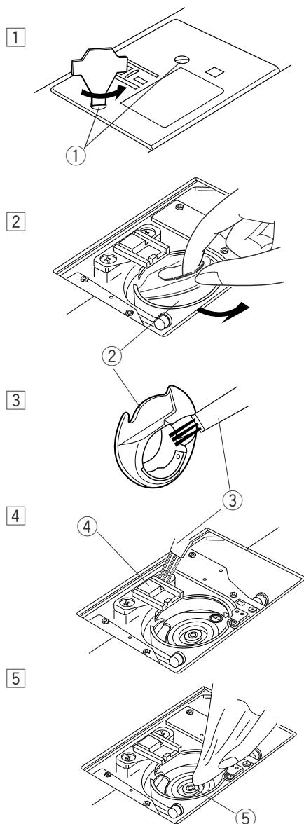
[1] Remove the presser foot and needle. Remove screw on the needle plate with the screwdriver.
