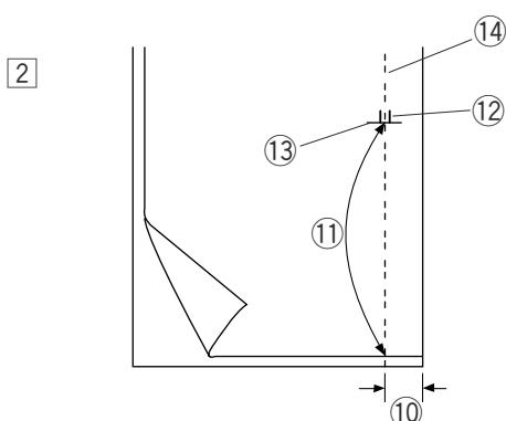
**2** Place the right (top) sides of the fabric together. Sew a bottom seam 5/8" (2 cm) from the right edge to the zipper bottom stop position. Sew a few stitches in reverse to lock. Increase the stitch length to "4", set needle thread tension to "1", and baste the entire length of the fabric.
