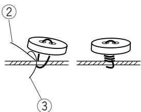
Unthread the needle. Adjust the stitch width to match it with the span of the holes in the button. Turn the handwheel to check if the needle enters into each hole in the button.
