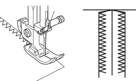
The zigzag stitch is used on the seam allowance to prevent fabric from fraying at raw edges.
