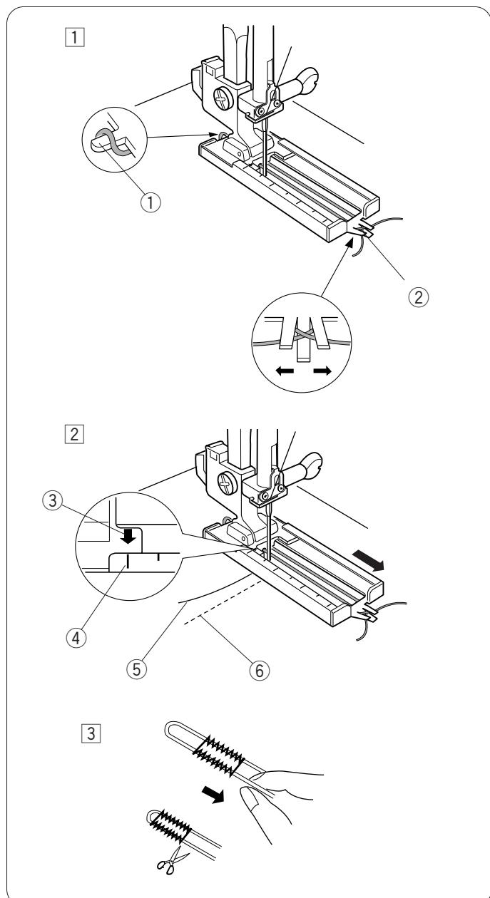
① With the buttonhole foot raised, hook the filler cord on the spur at the back of the foot.
