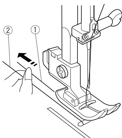
① Raise the presser foot and hold the needle thread lightly with your left hand.
