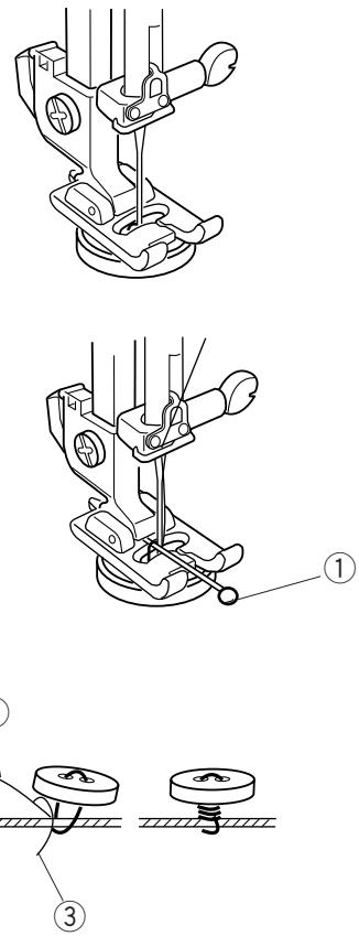
Unthread the needle. Adjust the stitch width to match it with the span of the holes in the button. Turn the handwheel to check if the needle enters into each hole in the button.
