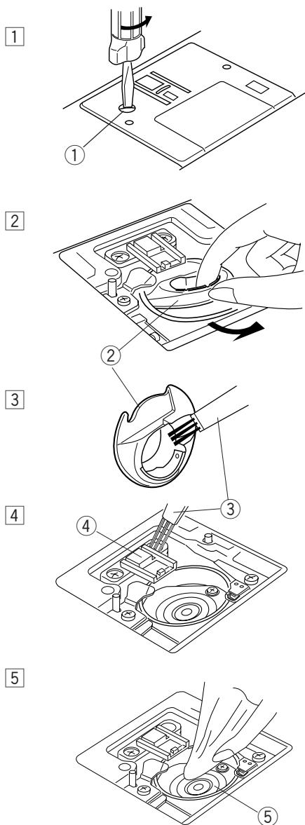
① Remove the presser foot and needle. Remove screw on the needle plate with the screwdriver.
