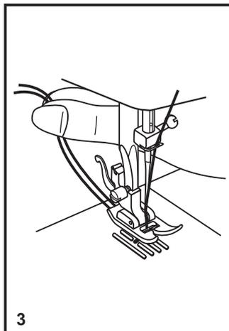
Gently pull on the upper thread to bring the bobbin thread up through the needle plate hole. (2)
