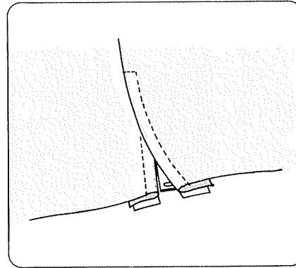
Pin or baste zipper tape to fabric and place it under the foot.
