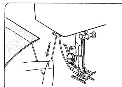
The threads are cut the proper length for starting the next seam.
