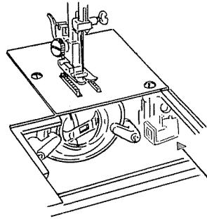
The drop feed lever is located in the hook area.
