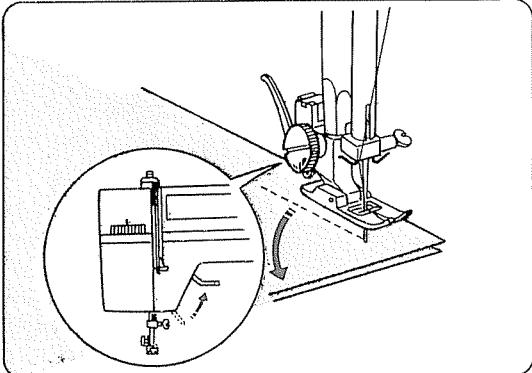
Stop the machine and turn the balance wheel toward you to bring the needle down into the fabrics.
