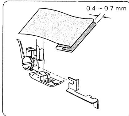
Fold up the desired amount and pin in place. Then fold the hem under the fabric as illustrated.
