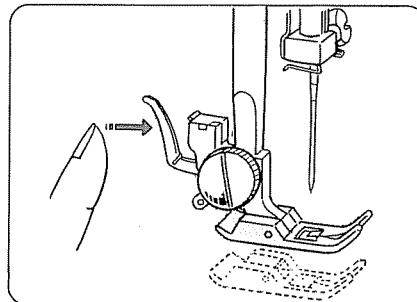
Press the lever on the back of the foot holder.
