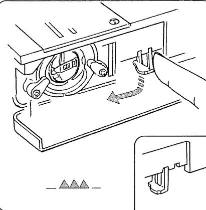
To raise the feed dogs, press down the lever and move it to the direction of arrow as illustrated.
