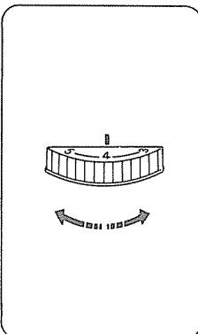
Set the desired number of the thread tension dial at setting mark.
