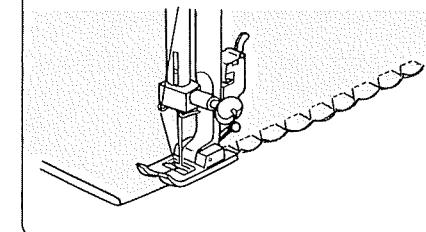
Place the folded edge along the slot of foot. The needle should fall off the edge of the fabric on the right forming a tuck.
