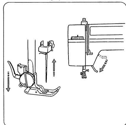
Raise the needle by turning the balance wheel toward you and lower the presser foot.
