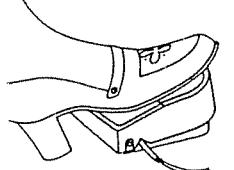
Sewing speed can be varied by the foot control. The harder you press on the control, the faster the machine runs.
