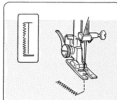
Set the zigzag width dial at "2", sew 5 stitches of bartack and raise the needle from the fabric.
