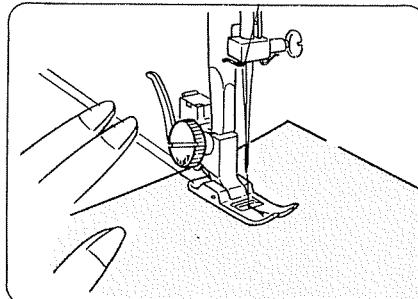
Raise the presser foot and position the fabric next to a stitching guide line on the needle plate.
