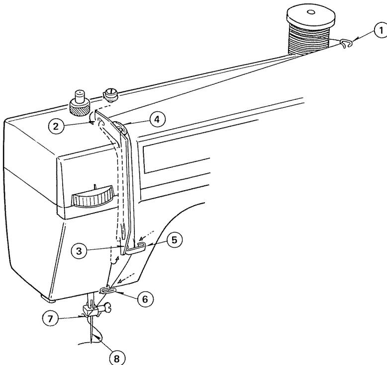
Raise the thread take-up lever to the highest point by turning the balance wheel towards you.
