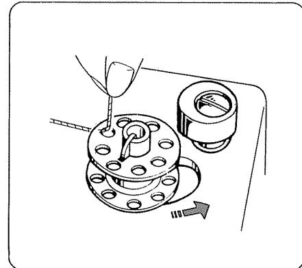
Draw thread from spool. Pass the thread through the top cover thread guide. Guide the thread around the bobbin winder thread guide. Insert the thread through the hole in the bobbin, threading from the inside to the outside. Put the bobbin on the bobbin winder spindle, and push it to the right.
