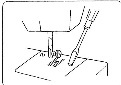
Remove the needle and the presser foot.
