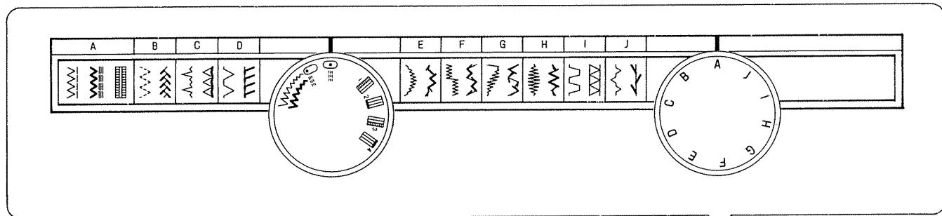
The stitch width for the zigzag stitches ( and ), the two needle positions (center and left) for the straight stitch and the triple strength stitch ( and ) and buttonhole stitching can be selected with the zigzag width dial.
