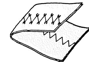
To obtain better zigzag stitches, the upper tension should be slightly weaker than in the case of straight sewing. The upper thread should appear slightly on the reverse side of the fabric.
