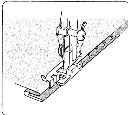
Raise the presser foot and place the fabric under the foot so that the soft fold rests against the wall of hem guide.
