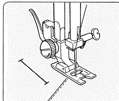
Set the zigzag width dial at "1". Slide both threads to the left. Lower the needle into the garment where the buttonhole is to start, and lower the foot.
