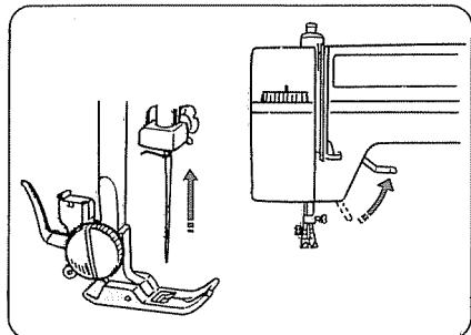
Turn the balance wheel toward you to raise the needle to its highest position.
