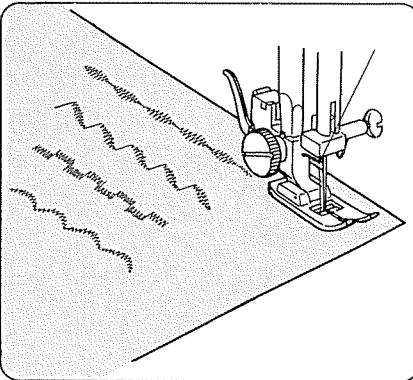
Sew a row of stitches and adjust the thread tension so the upper thread should appear on the reverse side of the fabric.
