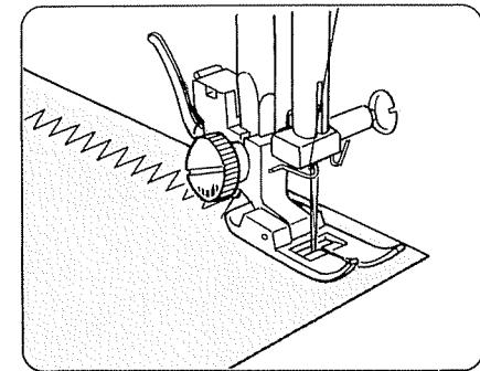
Simple zigzag stitching is widely used for overcasting, sewing on buttons etc.
