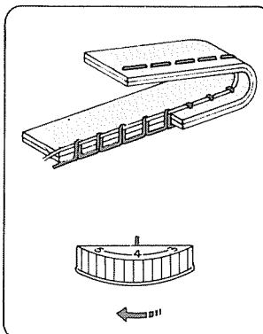
Loosen the needle thread tension by moving the dial to a lower number.
