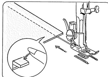
For fastening the ends of seams, press the reverse lever and sew several reverse stitches.
