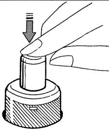
To increase pressure, push down the pressure regulator button until suitable pressure is obtained.
