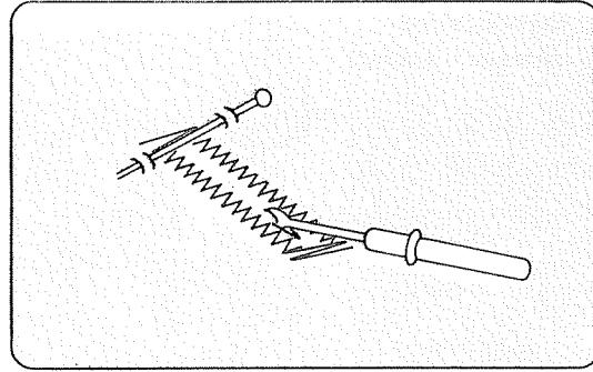
Remove the fabric from the machine and cut the sewing threads.
