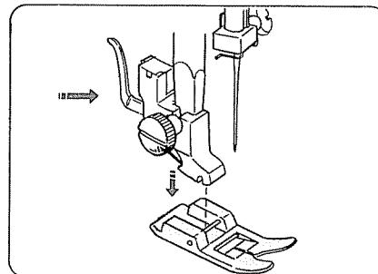
When attaching the presser foot, set the pressure regulator button at the depressed position to the bottom. Place the presser foot so the pin on the foot lies just under the groove of the foot holder. Lower the foot holder to lock the foot in place.
