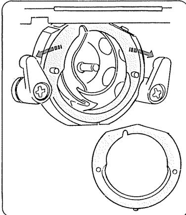
Open the hook race ring holders outside and remove the hook race ring.
