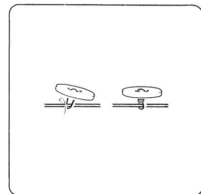
Set the zigzag width dial at "3~7". Align the both holes of the button with the slot of the foot and place the left hole of the button just below the needle point. Lower the foot and turn the pattern selector until the needle point comes just above the right hole of the button. Sew about five stitches and raise needle. Set the zigzag width dial at "3~7" again and sew a few stitches to lock thread.
