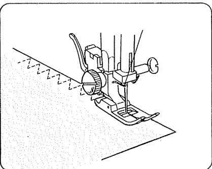
Place the fabric under the presser foot so that the edge will be slightly inside the right hand side of the presser foot. Guide the work so the right hand stitches fall at the edge of the fabric.
