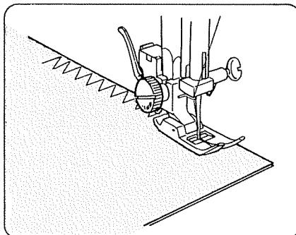
This type of stitch is used on the seam allowance to prevent fabrics from fraying at raw edges.
